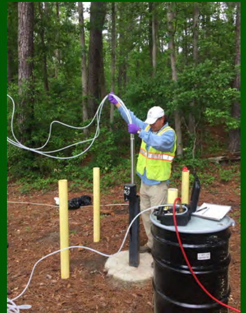
A Multistate Trust contractor is sampling groundwater from a monitoring well at the Kerr-McGee Chemical Corp – Navassa Superfund Site.
