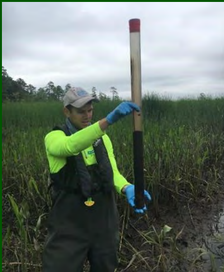
Multistate Trust contractors (above and right) use innovative, state-of-the-art sampling technology to cost effectively determine whether creosote contaminants are present in marsh sediments near the Brunswick River and Sturgeon Creek.
