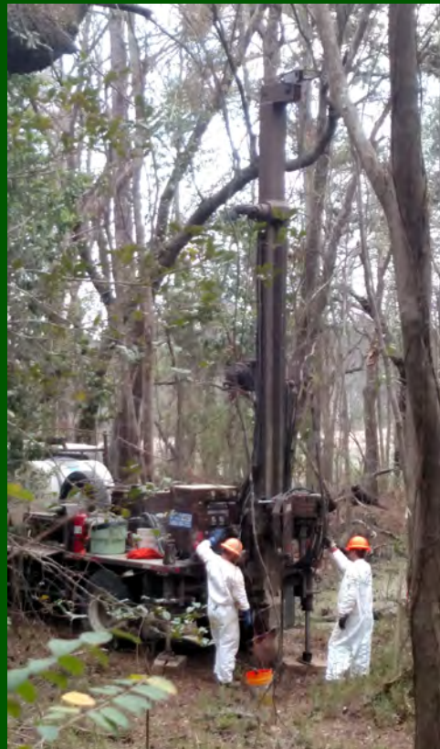
Multistate Trust contractors (above and right) use innovative, state-of-the-art sampling technology to cost effectively determine whether creosote contaminants are present in marsh sediments near the Brunswick River and Sturgeon Creek.
