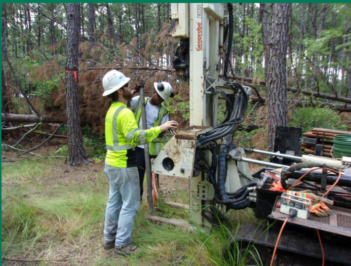
In June 2019, during soil sampling in the northern area of the Site, a Multistate Trust contractor's team (left) collects soil samples using a Geoprobe drilling rig. In May 2018, a Multistate Trust contractor's team (right) installs trenches to collect soil samples needed to evaluate subsurface conditions.
